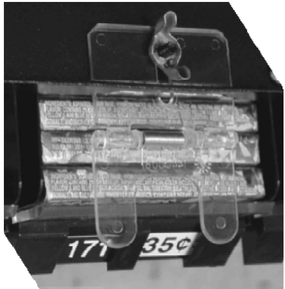
Figure 10: Correct gum and mint adjustment.
